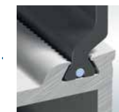
Cavity with insulbar® insulating profile inserted
